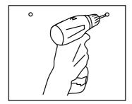
Drill using a 6-mm diameter drill bit (the correct diameter for the wall plugs supplied with the equipment).
