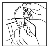
Position and connect the UVc lamp supplied in a protective shipping tube. Refer to the UVc lamp replacement maintenance procedure § VII – b) / fig: VII-4
