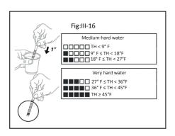
Measure the hardness of your water (TH) using the test strips supplied with the Komeo unit. To do this, immerse a test strip in a glass of tap water. Shake off the excess water, wait one minute, and then compare the colour to the scale shown above. This value will affect the antiscaling power setting you apply to Komeo (to perform this measurement, read the instructions on the test strips and read the value in °f) or in °e).
