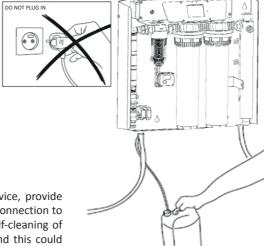
If there is no drain connection near the device, provide a 5-litre container for prefilter cleaning. For connection to the drain, provide a pipe connection (the self-cleaning of the prefilter is performed under pressure and this could cause the black pipe to come out of the drain connector).
