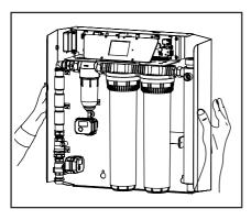
Place Komeo on its mounting points, check that the spacers are correctly positioned (between the machine and the wall), and tighten the four mounting screws.
