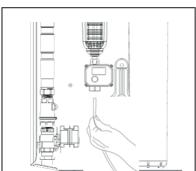
Position the hydraulic connection components you have chosen to connect Komeo to your installation.
