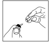
Remove the wall plugs from the screws and place the spacers between screw and wall plug. Choose appropriate wall plugs for the material and the weight of the machine (25 kg with water, with four mounting points).
