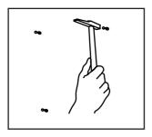
Insert the wall plugs in the holes, allowing the screw to protrude 5 mm beyond the spacer.
