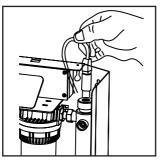
Once the hydraulic connection has been made, supply water by opening a valve upstream and a tap downstream to bleed out the air. Gradually close the tap as soon as water comes out of it. Check that Komeo and the connections are perfectly sealed.
